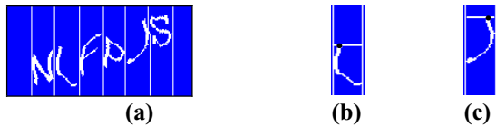
Fig 12. Recognising ‘L’ and ‘J’. (a) A segmented challenge. (b) The 2 nd segment was normalised and successfully recognised as ‘L’. (c) The 5 th segment was normalised and successfully recognised as ‘J’.
